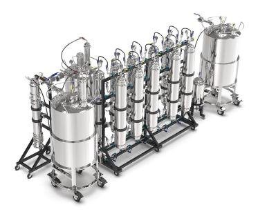
Closed-loop butane extraction removes the possibility of gas leaks, by containing all flammable solvents within a piece of commercial-grade extraction equipment. Closed-loop extraction is performed using third-party approved equipment at professional facilities with city government approval."
