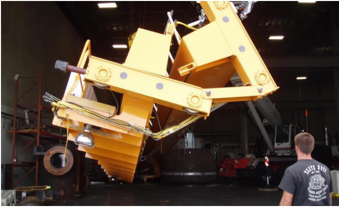
Derailed overhead crane. Picture credit r/CatastrophicFailure reddit group.
