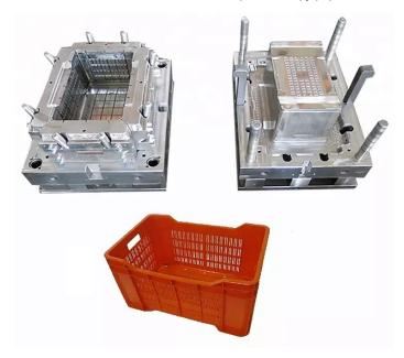
Injection molding has a slew of advantages. Plastic with different properties can be utilized, parts can be made of any color, the design tolerance is tight, high-volume orders are cost effective and the waste produced is not only small but can be re-ground and reused. The disadvantages are that to make a steel mold, the initial cost is relatively high. It can take about a month to complete the mold design and manufacture the custom mold.
