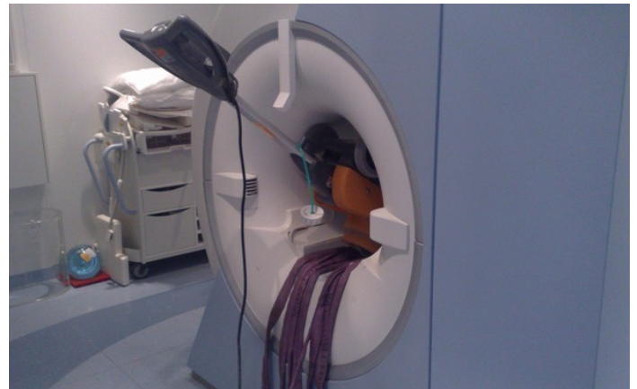
A floor polisher was attracted by an MRI. The polisher could only be removed by ramping down the magnetic field. Creative Commons Attribution-Share Alike 4.0 International, author: Xksev
