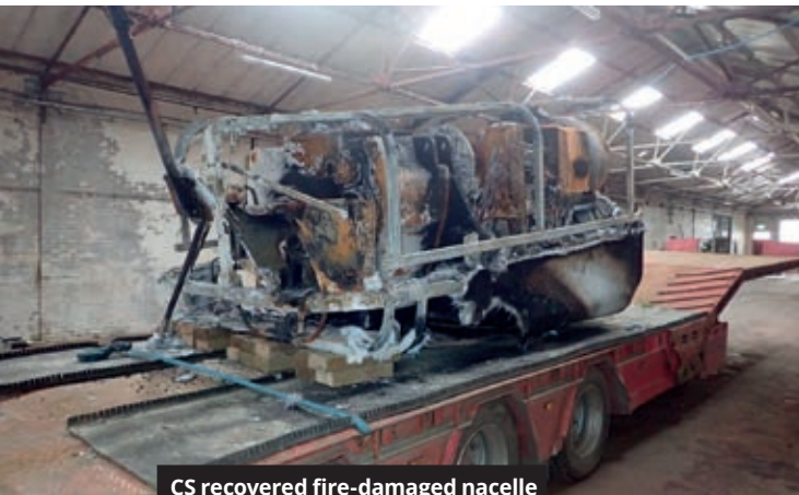
CS recovered fire-damaged nacelle
